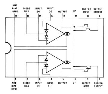
Figure 1. Top View Dual-In-Line and Small Outline Packages
