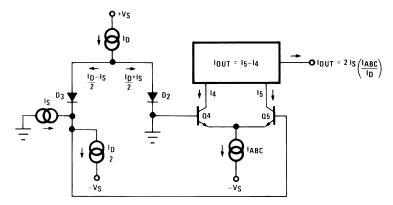
Figure 7. Linearizing Diodes
