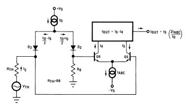
Figure 9. Equivalent VCA Input Circuit
