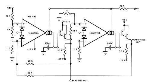
Figure 20. Voltage Controlled State Variable Filter
