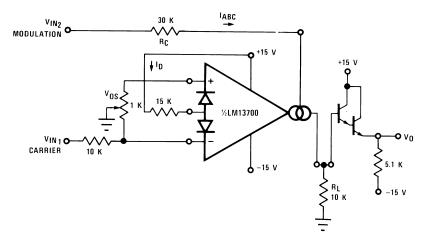
Figure 11. Amplitude Modulator
