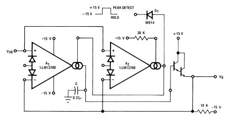
Figure 30. Peak Detector and Hold Circuit
