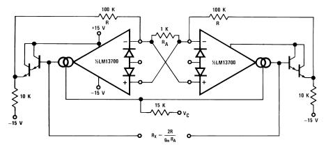
Figure 16. Floating Voltage Controlled Resistor
