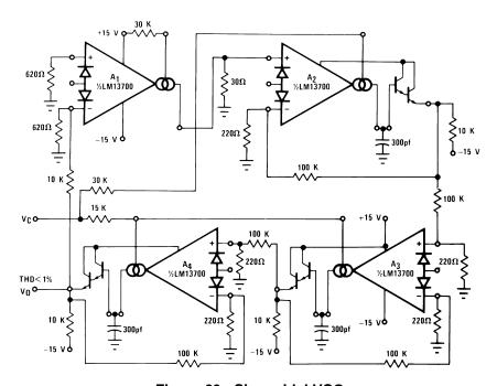
Figure 23. Sinusoidal VCO
