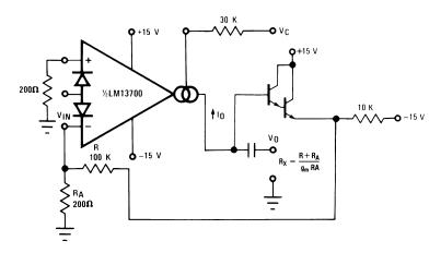
Figure 14. Voltage Controlled Resistor, Single-Ended
