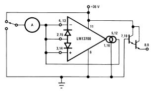
Figure 6. Differential Input Current Test Circuit
