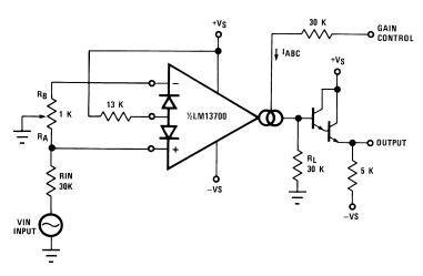
Figure 8. Voltage Controlled Amplifier
