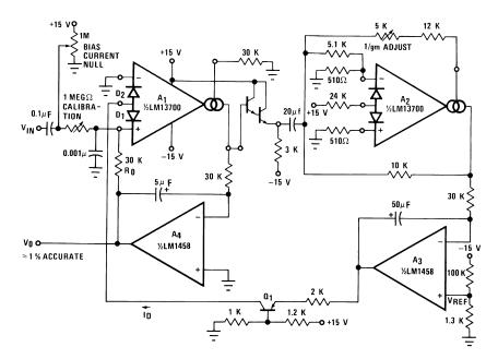
Figure 33. True RMS Converter
