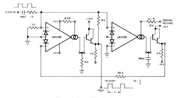
Figure 35. Pulse Width Modulator
