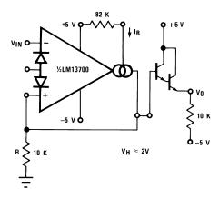
Figure 28. Schmitt Trigger
