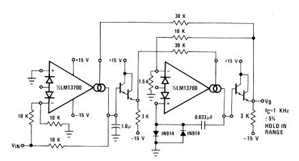
Figure 27. Phase Lock Loop
