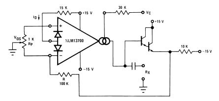
Figure 15. Voltage Controlled Resistor with Linearizing Diodes
