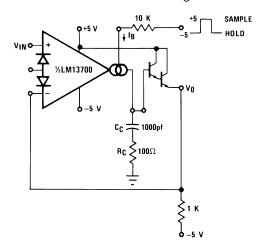
Figure 31. Sample-Hold Circuit
