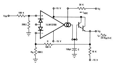
Figure 17. Voltage Controlled Low-Pass Filter
